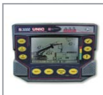
SLI pre-programmed with fly jib and searcher hook data
