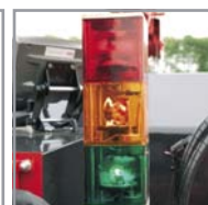
Overload warning lamps + auto stop + alarm
